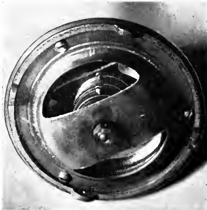
FIG. 34.—SWEDISH-AMERICAN TRANSMITTER, CAP REMOVED.
